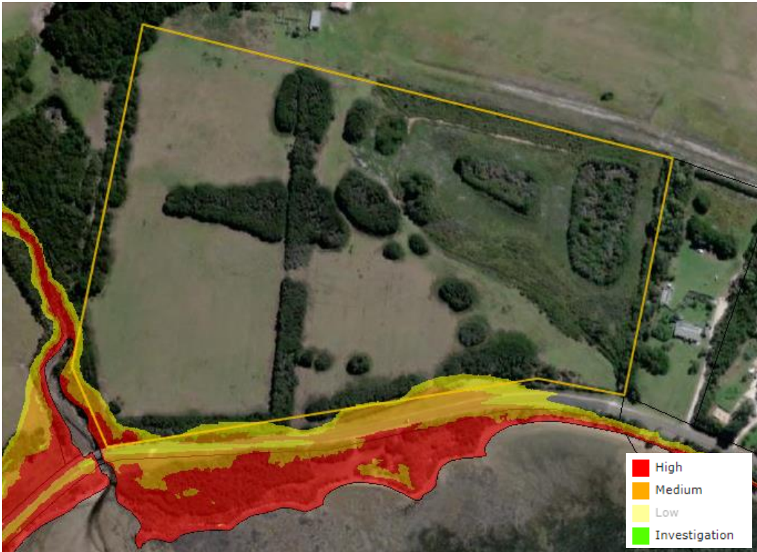
Figure 4 Coastal inundation hazard bands
