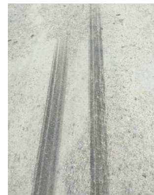
Aircraft skid marks shows hardness of stabilised pavement prior to seal coats being applied
