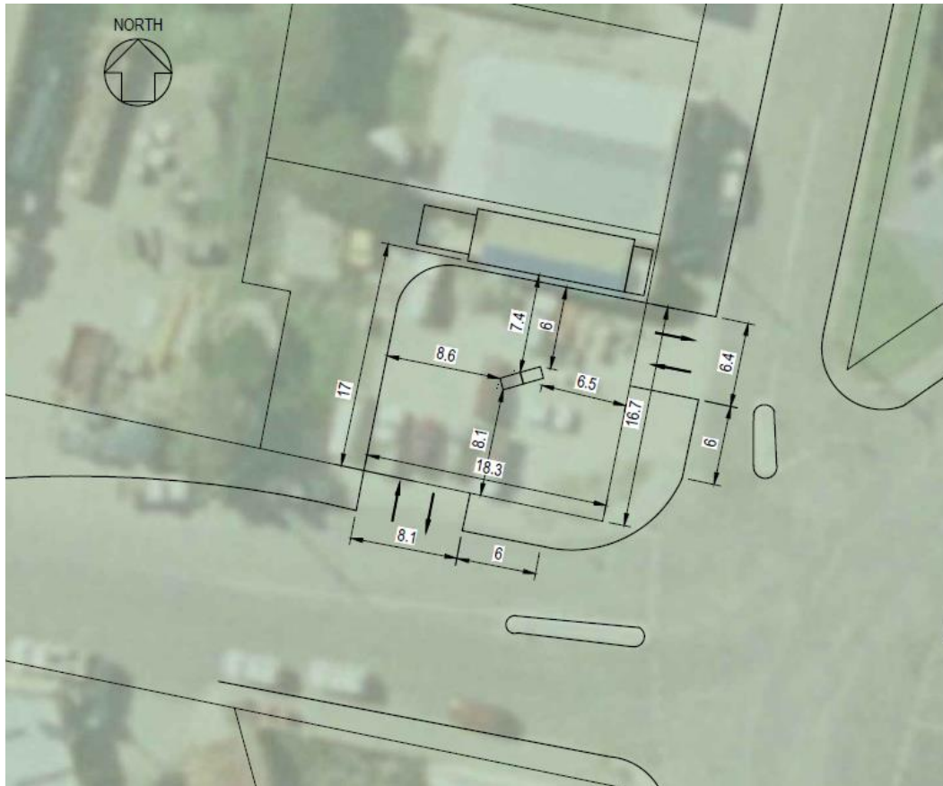
Drawing No. LN19136-P03 dated 06/06/2019 by Pitt & Sherry: showing the relocated bowzers.
