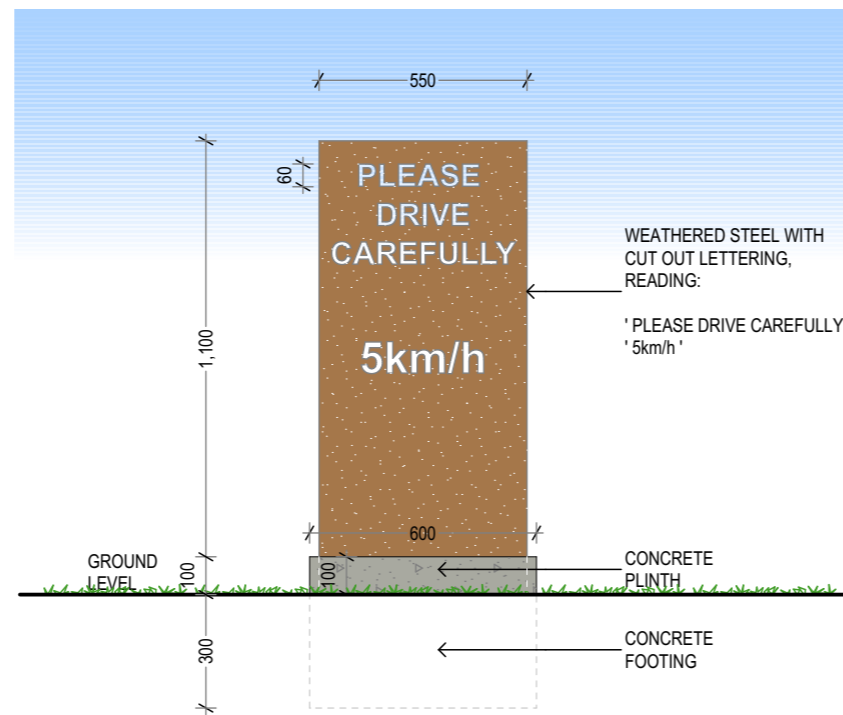
SPEED LIMIT BEACON DETAIL 1 1:20
